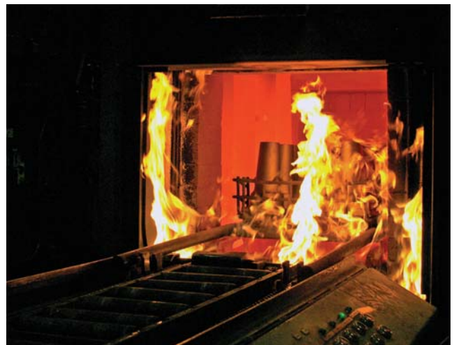
Load of parts entering an atmosphere furnace
